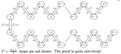
Gusev (Lower bounds for the length of reset words in Eulerian automata, Reachability Problems, LNCS 6945, 180–190 (2011)) has constructed another series of Eulerian synchronizing automata with n states and 2 input letters whose reset threshold is  $\frac{n^2-3n+4}{2}$ . The construction and the proof are elegant. Define the automaton  $\mathcal{M}_n$  (from Matricaria) on the state set  $\{1, 2, \ldots, n\}$ , where  $n \geq 5$  is odd, in which a and b act as follows:
