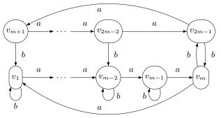
The automata in the series have subsets that require words of length as big as  $m^2 + O(m)$  in order to be extended.
