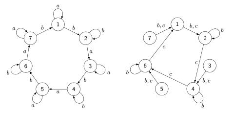
The automaton  $\mathscr{M}_7$  and the automaton induced by the actions of b and c = ab
